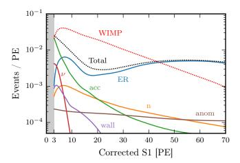
FIG. 3: Background model in the fiducial mass in a reference region between the NR median and  $-2\sigma$  quantile in cS2<sub>b</sub>, projected onto cS1. Solid lines show that the expected number of events from individual components listed in Table I; the labels match the abbreviations shown in the table. The dotted black line *Total* shows the total background model, the dotted red line *WIMP* shows an  $m = 50 \text{ GeV/c}^2$ ,  $\sigma = 10^{-46} \text{cm}^2$  WIMP signal for comparison.
