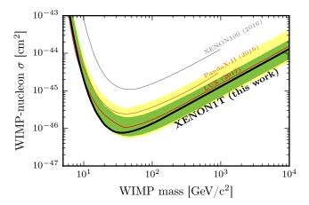
FIG. 4: The spin-independent WIMP-nucleon cross section limits as a function of WIMP mass at 90% confidence level (black) for this run of XENON1T. In green and yellow are the 1- and  $2\sigma$  sensitivity bands. Results from LUX [27] (red), PandaX-II [28] (brown), and XENON100 [23] (gray) are shown for reference.
