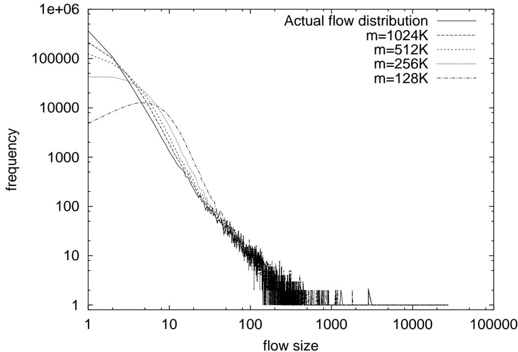
The distribution of flow sizes and raw counter values (both  $x$  and  $y$  axes are in log-scale).  $m = \text{number of counters}$ .
