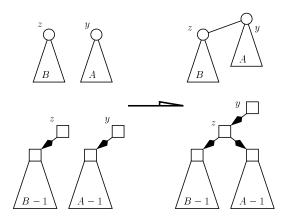
Figure 2. The effect of one linking. Circular nodes correspond to the general representation and square ones to the binary representation.
