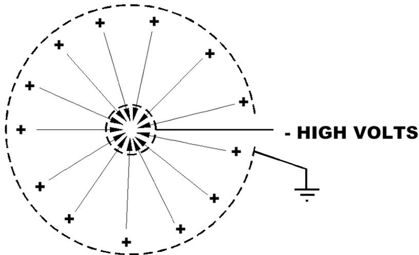
Figure 1. A Hirsch-Farnsworth "fusor" ion accelerator.
