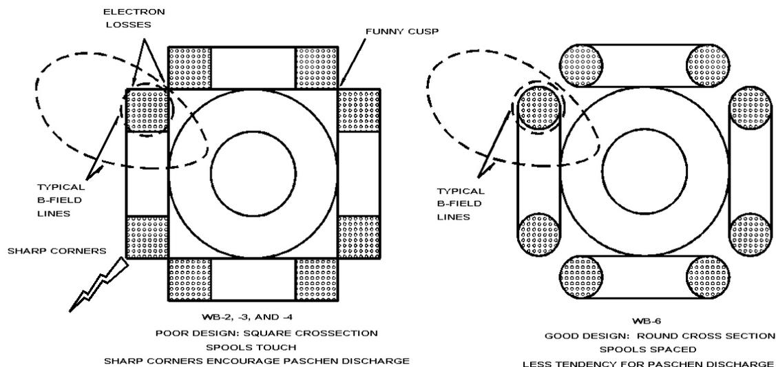
Figure 6. The flawed design of WB2, 3, and 4 was replaced by the good design of WB-6, shown on the right. This greatly reduced electron losses, and allowed the machine to validate the concept.
