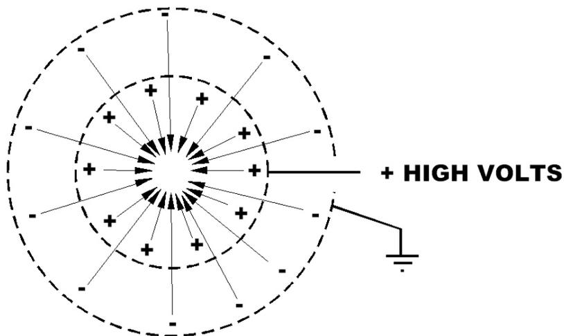
Figure 2. An Elmore-Tuck-Watson electron accelerator with ion-accelerating central potential well.
