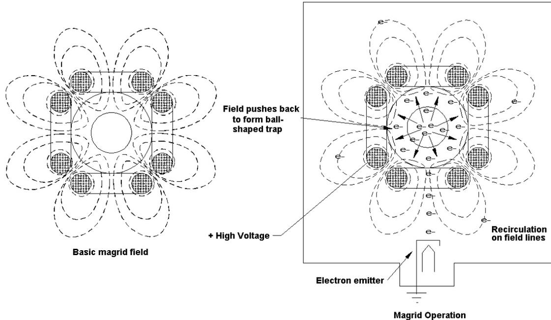
**Figure 3. Magrid operation and formation of the diamagnetic trap “ball”.**
