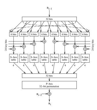
Figure 15: One iteration of the inner loop of DES. The  $\oplus$  symbols indicate exclusive-or operations.
