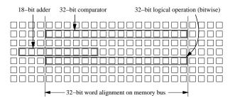
Figure 3: Typical natural layouts of multi-bit functions.
