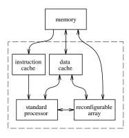
Figure 1: Basic Garp block diagram.
