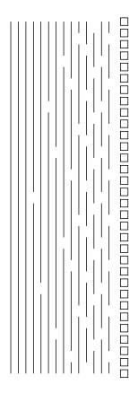
Figure 8: The pattern of vertical wires (V wires) in a single column of 32 rows. Each line drawn actually represents a pair of wires (2 bits).
