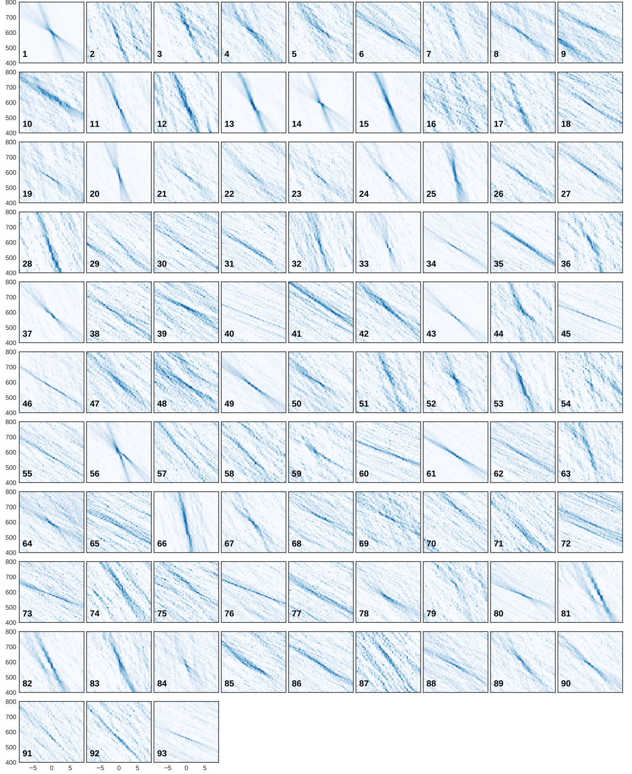
Figure 9. Dedispersion verification plots of all pulses. All panels have the same scale. The horizontal axes are time of arrival extrapolated to the same frequency in milliseconds, and the vertical axes are DMs in the usual \text{pc cm}^{-3} . The colors indicate flux density after incoherent dedispersion and the colors are scaled individually for each plot. A light color (high value) near the center of the panel indicate a close-to-expectation DM and TOA.
